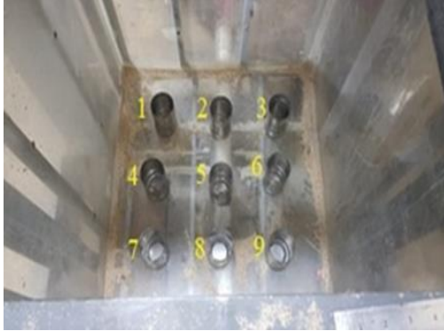
Fig. 6 Locations of molds used to measure sand density
