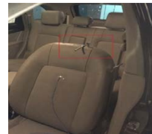
Fig. 5 A position of the microphone : a position at the neck of the backrest of the cushion beside the driver
