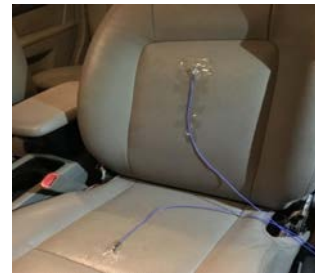
Fig. 3 Two positions of the vibration sensors : the backrest and the bottom seat of the cushion beside the driver
