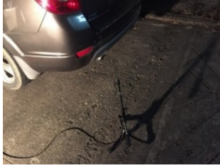
Fig. 7 A position of the microphone : a position at the rear of the exhaust pipe with a 45-degree angle to that pipe and a 0.5-meter far distance
