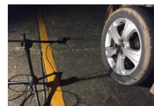
Fig. 6 A position of the microphone : a position beside the front wheel with 0.5-meter far distance
