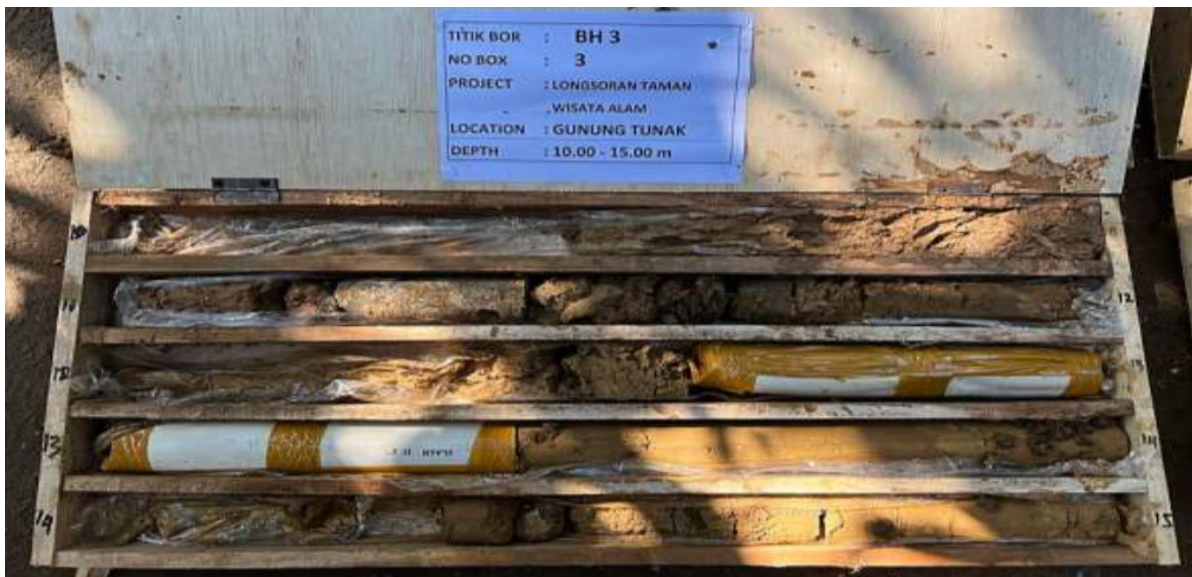
Fig. 2 Soil samples in wooden core boxes
