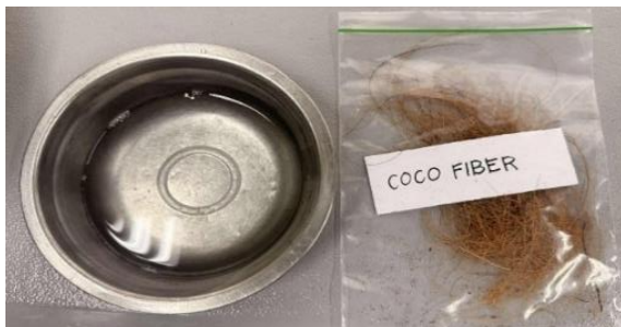
Fig. 6 Alkaline solution and coconut fiber
