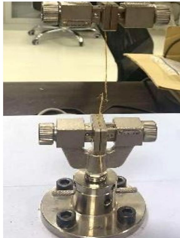
Fig. 8 Fibers after the tensile strength testing
