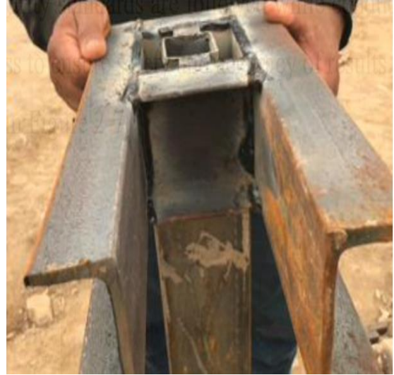
b) C-section for Eccentric Columns
