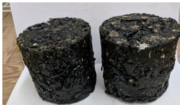
Fig. 8. Macrosections of fractured specimen surfaces: (a) specimen with cellulose fiber, (b) specimen with PET fiber (arrows indicate zones of fiber and pore accumulation).
