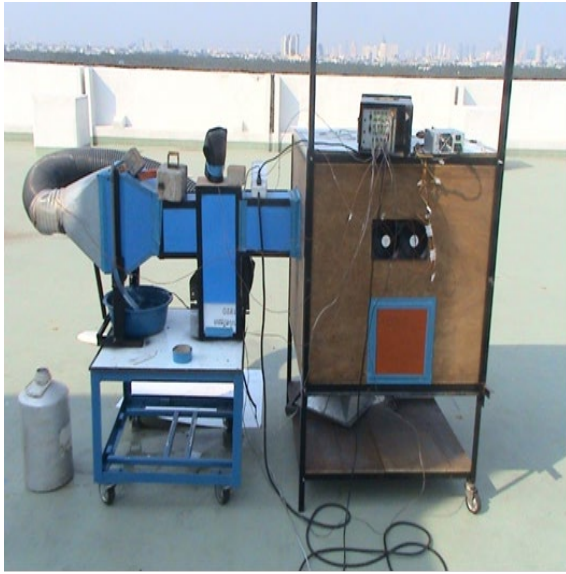
Fig.1 Experimental setup of the hybrid evaporative cooling system integrated with heat pipes
