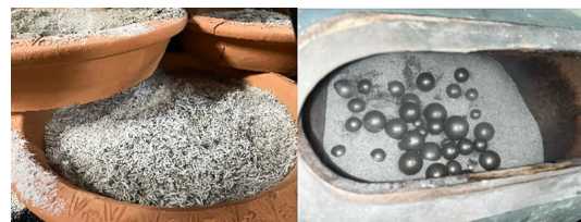
Fig.1 Burning rice husk ash and rice husk ash mashed ball mill grinding machine
