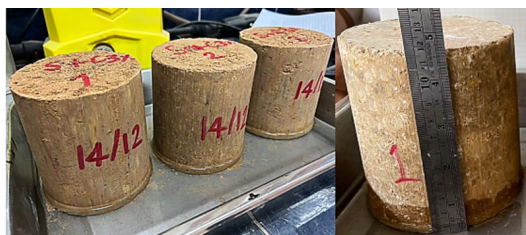
Fig. 2 Capillary rise test conducted on specimens
