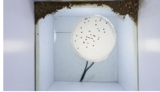
Fig. 6 Raw Image of Particles Retained in No. 10 Sieve
