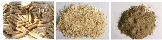
Fig. 1 Preparation of the corn cob pore-forming additive for pellet fabrication: (a) raw corn cob residues, (b) milled corn cob particles, and (c) sieved corn cob fraction used for mixing with clay.
