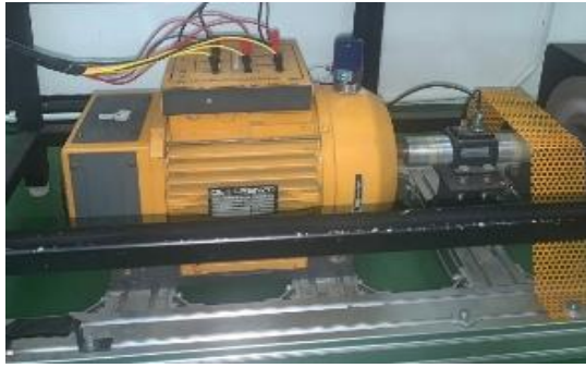
Fig.1 The synchronous motor used in the experiment.
