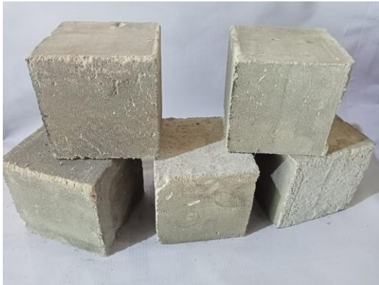
Fig.2 Cellular Lightweight Concrete (CLC) mortar
