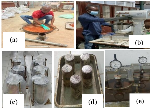
Fig. 2 Sample preparation: (a) Manual mixing (unstabilized); (b) Mechanical mixing (stabilized); (c) 7-day sealed curing (CBR); (d) 7-day sealed curing (UCS); (e) 4-day soaking /swelling measurement
