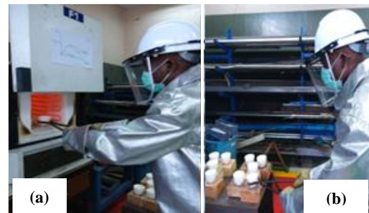
Fig. 1 Thermal activation of kaolin clay: (a) Muffle furnace used for calcination. (b) Cooled crucibles containing the resulting metakaolin after heating.
