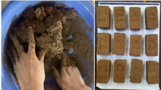
Fig. 2 Manual mixing of raw materials for clay bricks.
