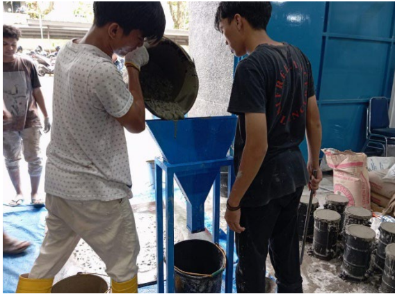
Fig. 10 V funnel test
