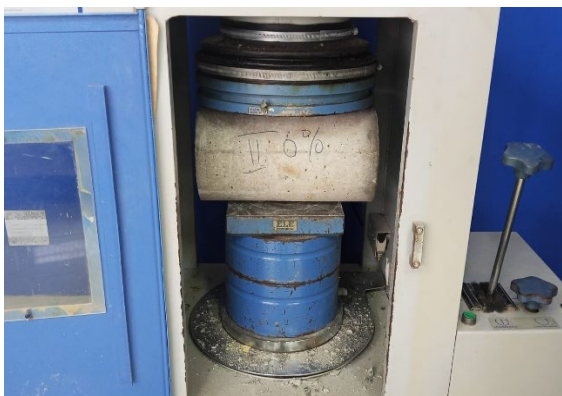
Fig.13 Tensile test on cylindrical specimen
