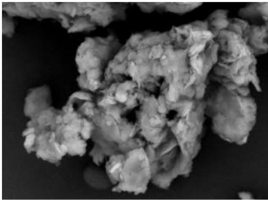
Fig.4. The microstructure of concrete sample 1 on 250 times magnification
