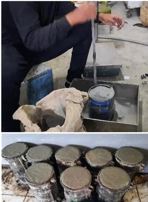
Fig.2 The molding process of concrete materials
