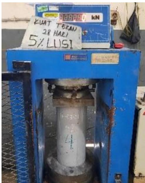
Fig.3 Concrete compression machine
