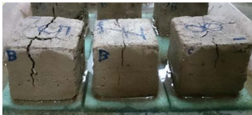
Fig. 14 The samples without reinforcement after soaked in the water for 24 hours.
