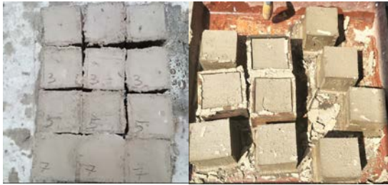
Fig.3 Samples preparation for unconfined compressive strength tests.
