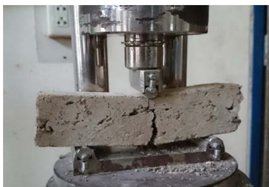
Fig.4 Flexural strength test of the specimen.
