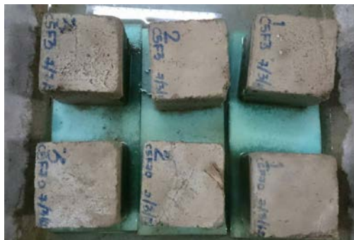
Fig. 15 The samples reinforced by water hyacinth fiber soaked in the water for 7 days.
