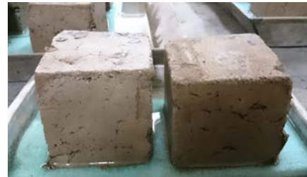
Fig.5 The specimens conducted on capillary rise tests.
