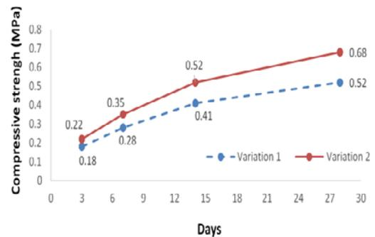
Fig. 6. Compressive strength of CLC
