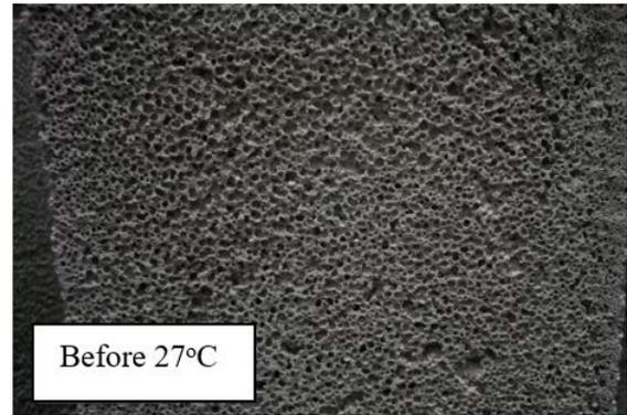
Fig. 9 CLC block pores before exposure high temperature
