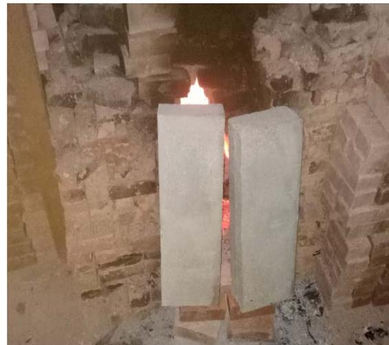
Fig. 4 Process of heating CLC block in the furnace
