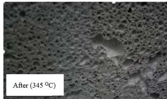
Fig. 10 CLC block pores after exposed high temperature.
