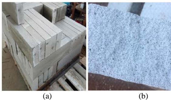
Fig. 1 (a) The Cellular Lightweight Concrete (CLC) block, (b) and the texture of CLC [8].
