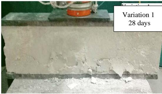
Fig 7. The compressive test on specimen Variation 1
