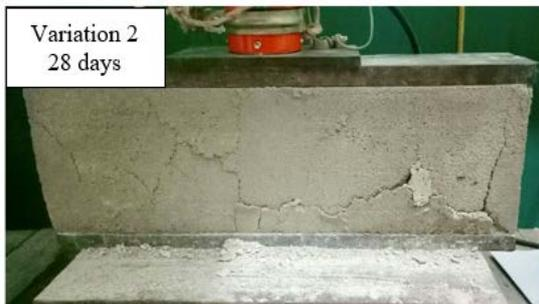
Fig 8. The compressive test on specimen Variation 2
