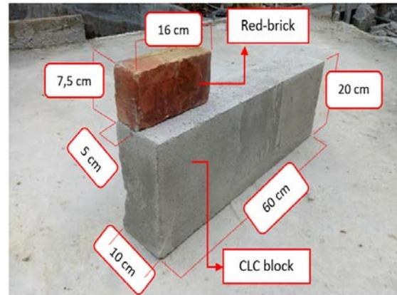
Fig. 2 Dimension of red-brick and Cellular Lightweight Concrete (CLC)
