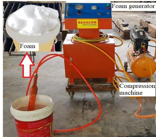
Fig. 3 The process of making foam using a foam generator
