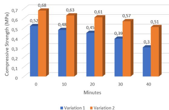
Fig. 11 The performance of CLC on 28 days after exposed high temperature during 0 to 40 minutes
