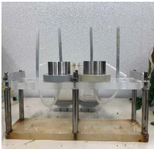
Fig. 2 Laboratory experiment of the bio-cementation of slope soil.
