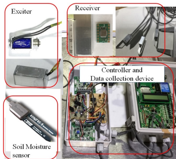
Fig.8 Elastic wave monitoring devices, which can automatically generate elastic wave and measure wave signal.
