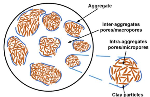
Fig. 8 The structure of aggregated soil [39].
