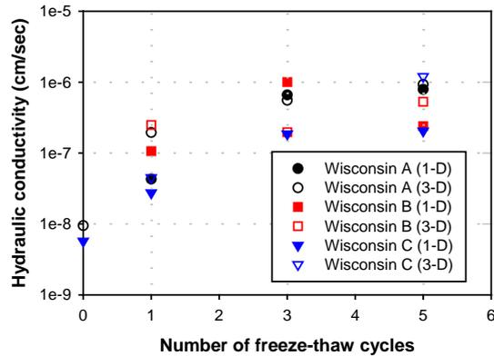
Fig. 4 Effect of F-T cycles on hydraulic conductivity [20].
