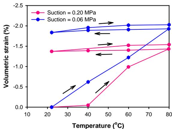
Fig. 9 Volumetric strain due to thermal cycling [40].
