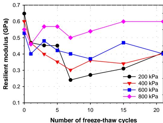
Fig. 6 Effect of F-T cycles on resilient modulus [26].
