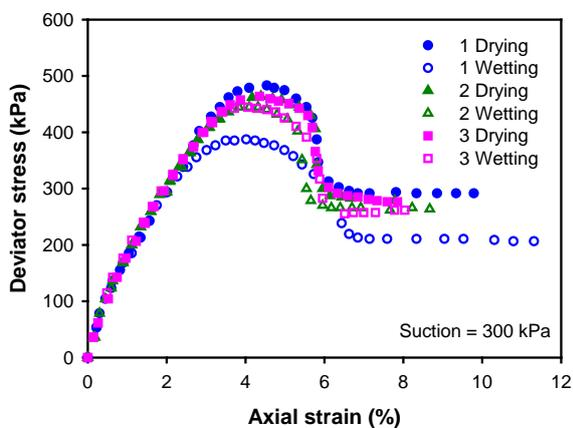
Fig. 12 Stress-strain relations during three W-D cycles [51].
