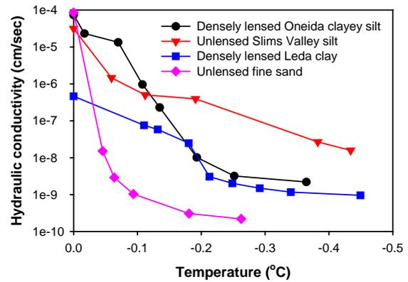
Fig. 1 Hydraulic conductivity of frozen soils [9].
