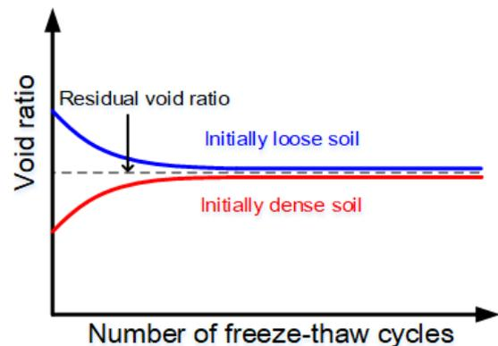
Fig. 3 Effect of F-T cycles on void ratio.
