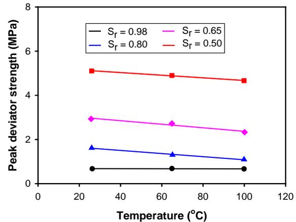
Fig. 11 Strength reduction due to temperature [48].
