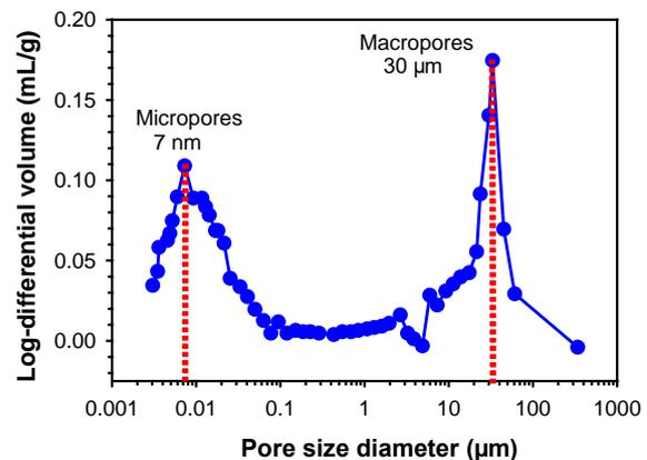
Fig. 7 Pore size distribution of an expansive soil [31].
