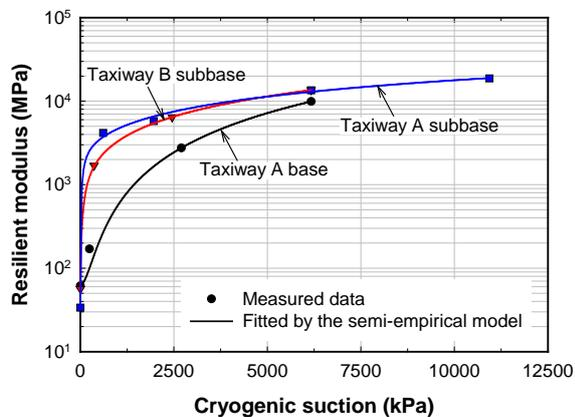
Fig. 2 Prediction of  $M_R$  of frozen saturated soils using the SFCC [15].
