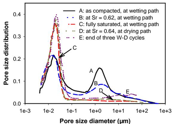
Fig. 10 Evolution of microstructure due to W-D cycles [46].
