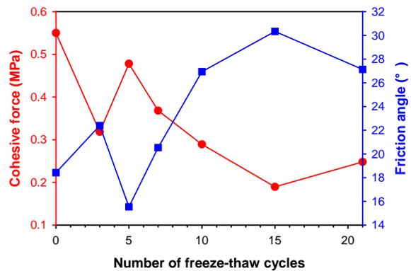
Fig. 5 Effect of F-T cycles on shear strength [27].
