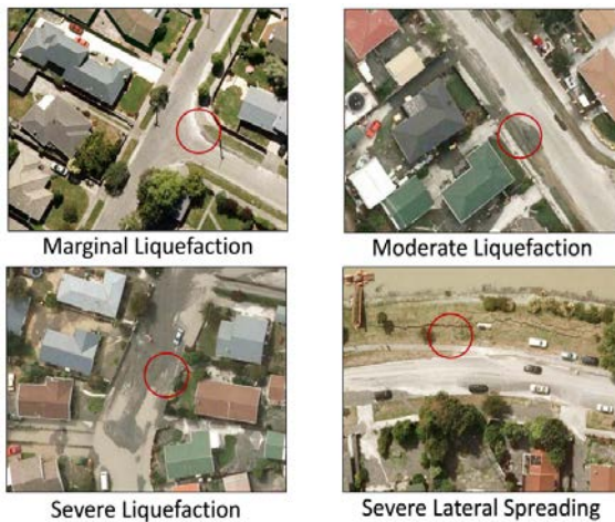
Fig. 1 Bird-eye observed liquefaction [8]
