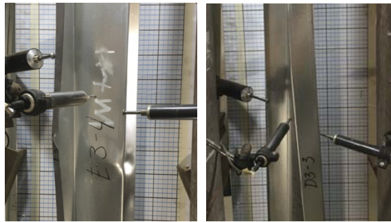
Fig. 4 Failure due to torsional-flexural buckling (right) and distortional buckling (left)
