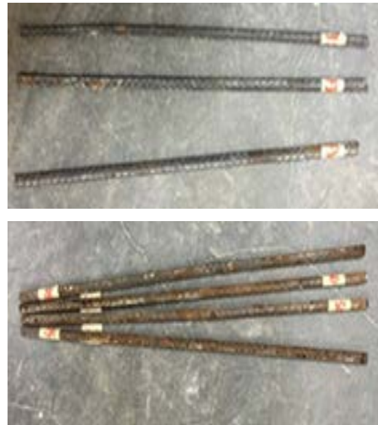
Fig. 7 Steel bars from “freshwater beam” (top), steel bars from “seawater beam” (bottom)
