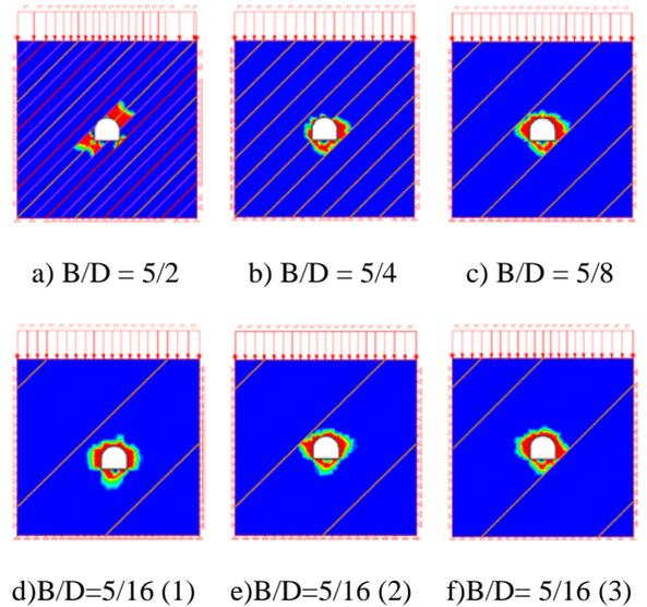
Fig.3 Failure zones of rock mass around roadways with the changing ratio of B/D
