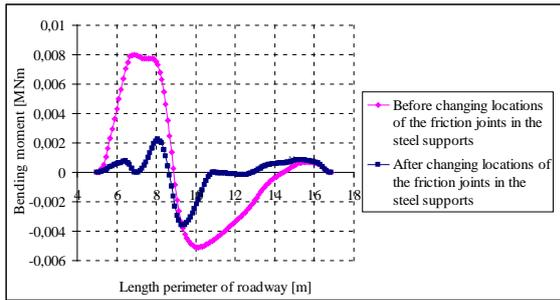
Fig.9 Bending moment in the steel supports in case of  $B/D = 5/8$
