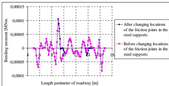
Fig.10 Bending moment in the steel supports in case of  $B/D = 5/16 (1)$
