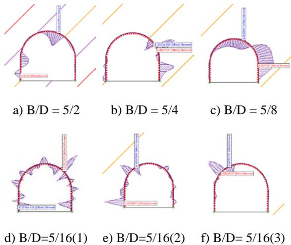
Fig.4 Graphics of bending moment in the supports with the varies thickness of rock mass layers
