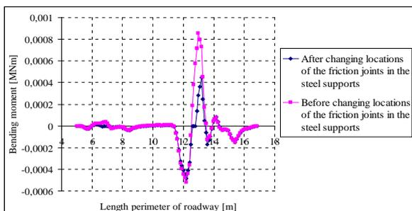
Fig.12 Bending moment in the steel supports in case of  $B/D = 5/16 (3)$
