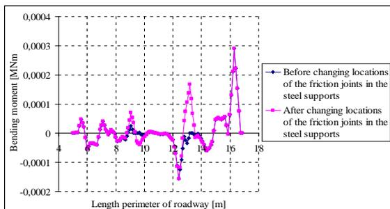
Fig.11 Bending moment in the steel supports in case of  $B/D = 5/16 (2)$
