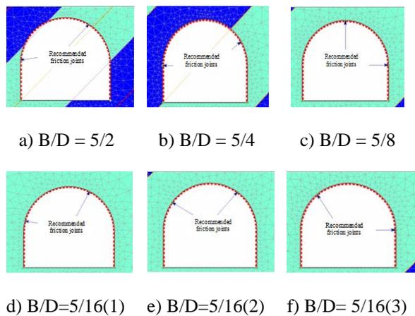
Fig.5 Recommendation of friction joints between arc and sidewalls of the steel supports in the roadways
