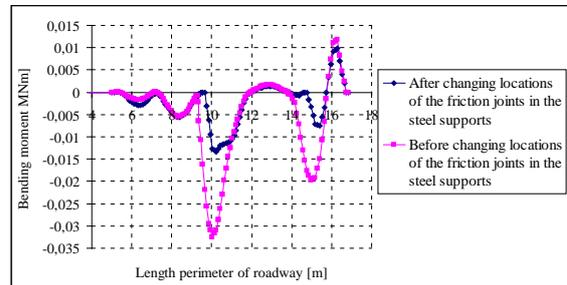
Fig.7 Bending moment in the steel supports in case of B/D = 5/2
