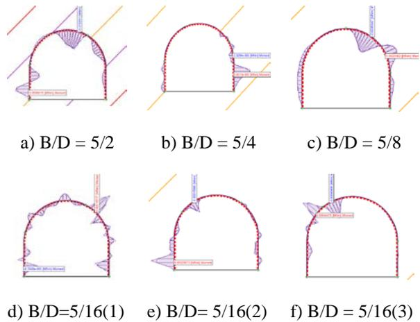
Fig.6 Graphics of bending moment in the steel supports and other locations of the friction joints
