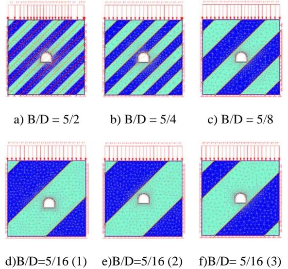
Fig.2 Models by Phase2 with the alteration of B/D
