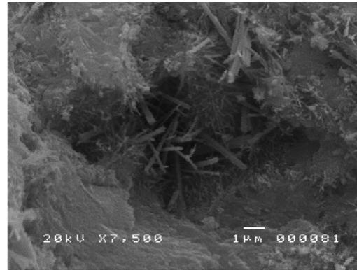
Fig. 4 SEM of mortar with 15% HDPE (15HDPE)
