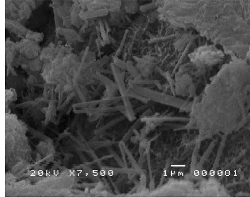
Fig. 3 SEM of mortar with 10% HDPE (10HDPE)
