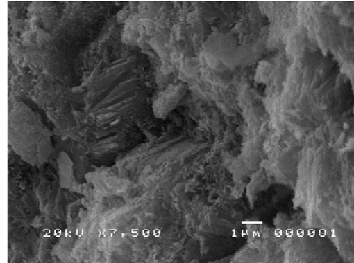
Fig. 5 SEM of mortar with 20% HDPE (20HDPE)
