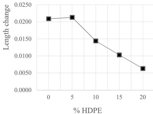
Fig. 6 Length change in mortar with varying HDPE
