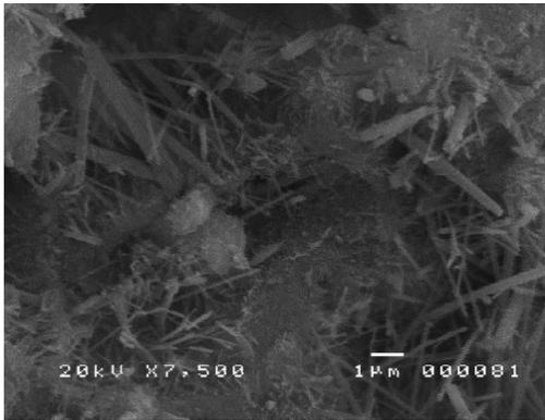
Fig. 2 SEM of mortar with 5% HDPE (05HDPE)
