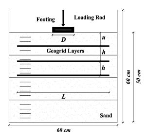
Fig. 5 Geometric parameters of geogid-reinforced sand.
