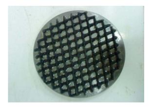
Fig. 3 Rough base of Circular footing.
