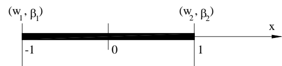
Fig.3 Isoparametric beam element not considering transverse shear strain
