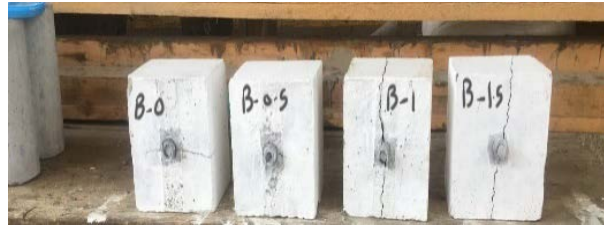
Fig. 6. Modes of failure - group B
