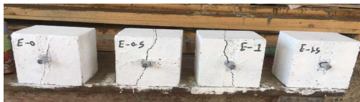
Fig. 12. Modes of failure - group E
