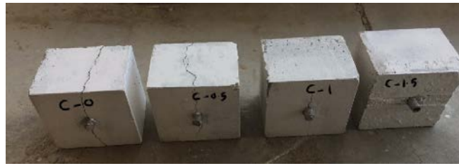
Fig. 8. Modes of failure - group C
