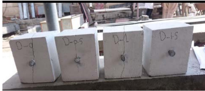
Fig. 10. Modes of failure - group D
