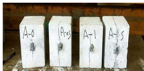
Fig. 4. Modes of failure - Group A
