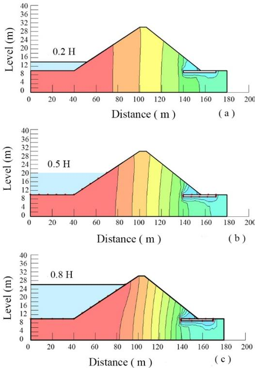
Fig. 5 Three different upstream water level
