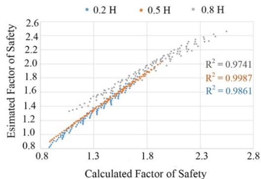
Fig.12 Estimated Fs versus Calculated FS
