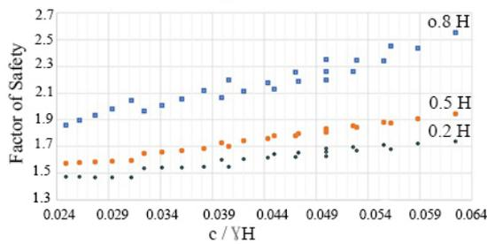
Fig.9 Factor of Safety VS  $\frac{c}{\gamma H}$
