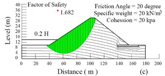
Fig. 6 Samples of different soil properties with the same upstream water level with different FS
