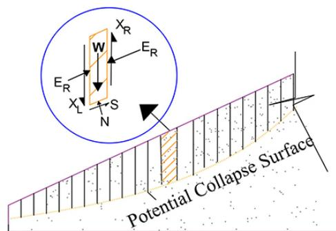
Fig.1 Basic of slice forces (Redrawing from [2], [5])
