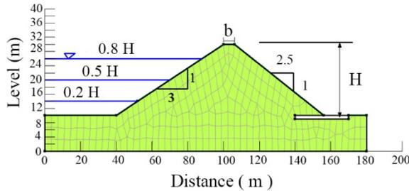
Fig. 4 Geometrical dimensions of studied dam
