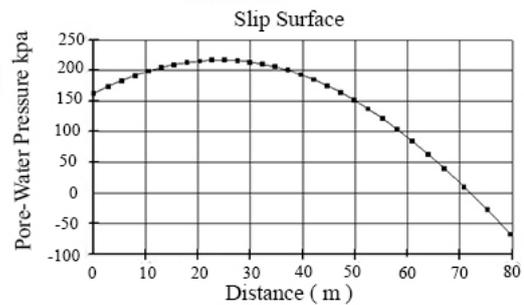
Fig. 7 Pore Water pressure related distance
