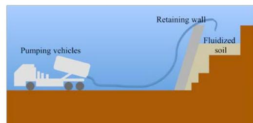
Fig. 2 The backfilling of the retaining wall
