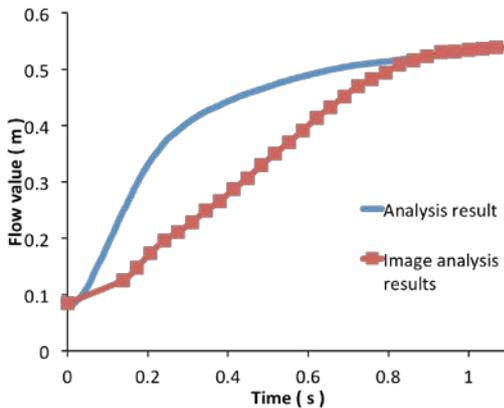
Fig. 11 Simulated flow-ability for the fluidization treated soil (B)
