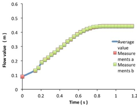
Fig. 5 Flow behavior of the fluidization treated soil (A) by image analysis
