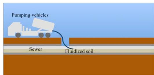
Fig. 1 Pumping of underground space
