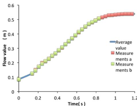
Fig. 6 Flow behavior of the fluidization treated soil (A) by image analysis
