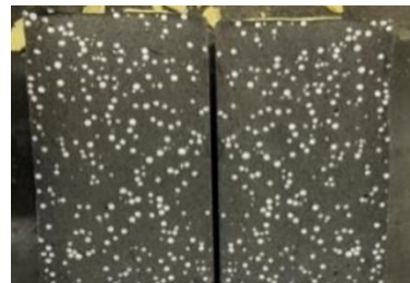
Fig.8 Cross section of the specimen after splitting tensile testing
