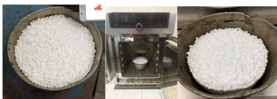
Fig.2 The heat treatment process of EPS beads.
