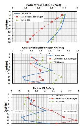
Fig.4a Results of the comparison of different ratios of cyclic resistance based on different methods
