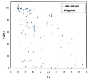
Fig.9 Graph of safety factor showing changes in the behavior of Idriss and Boulanger's method with probability using the GP software
