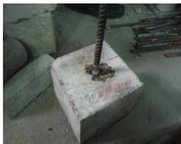
Fig.8: 12 mm re-bars slippage behavior.
