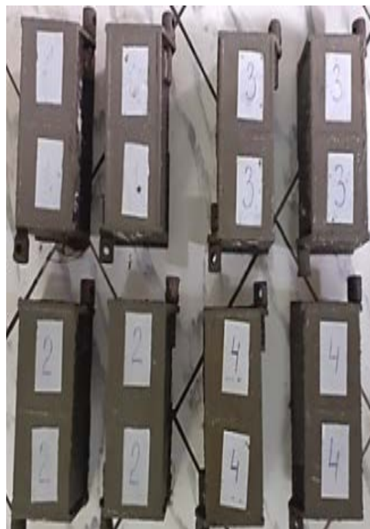
Fig. 1 Accomplished samples-cubes of concrete mix with the addition of man-made waste: 1 - control sample, without additives; 2 – with the addition of 20% of man-made waste; 3 – with the addition of 15% of man-made waste; 4 – with the addition of 10% of man-made waste
