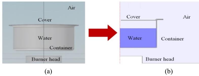
Fig. 5 The numerical model that used in the simulation (a) 3-D model and (b) 2-D axial symmetry model.
