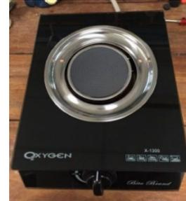
Fig. 1 Infrared gas stove which is used in the experiment.
