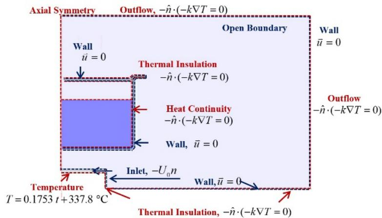
Fig. 6 Boundary conditions for numerical analysis.
