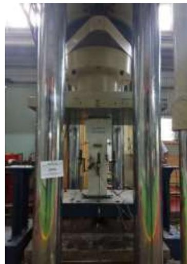
Fig. 2 Photograph of UTM with a specimen ready for testing. Source: authors
