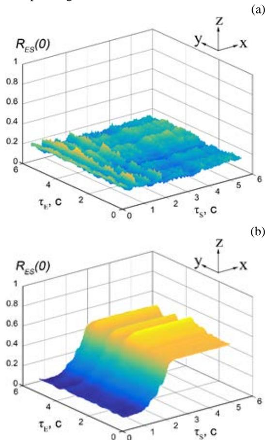
Fig.4 Measured CCC maximum as a function of time interval shift (a) – without a deposit, (b) – Bystryansky gas condensate deposit.
