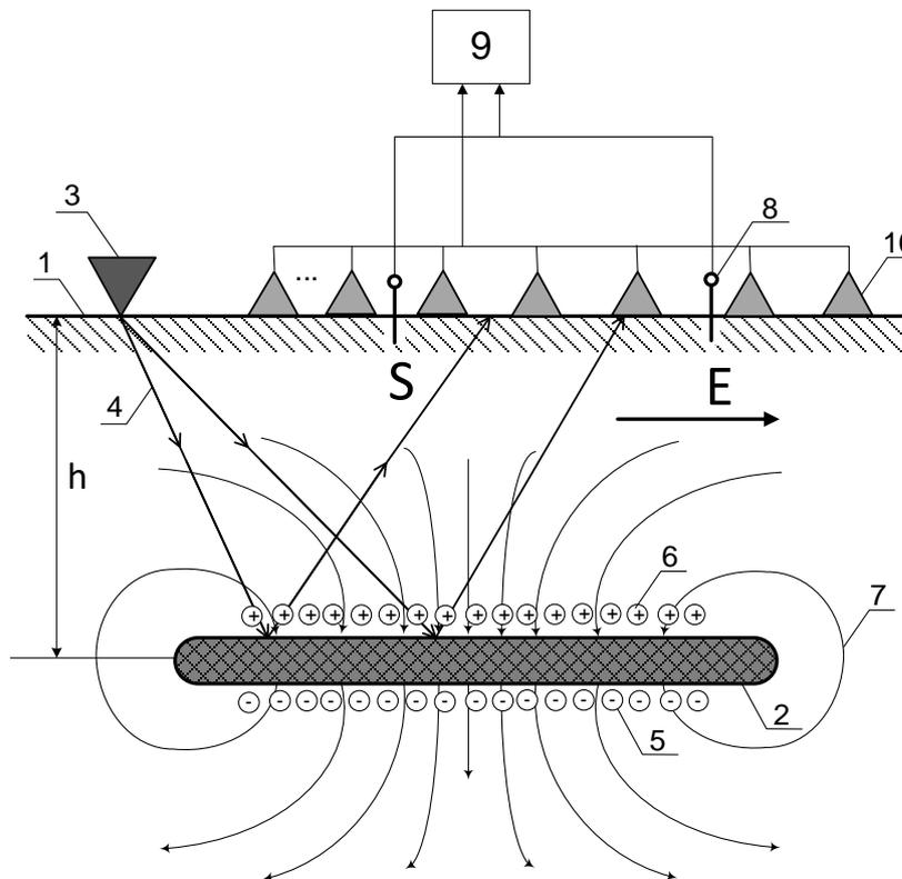
Fig.3 Installation diagram: 1 – ground level, 2 – productive seam, 3 – KEM-4 seismic oscillator, 4 - incident and reflected seismic waves, 5, 6 –charges at deposit boundaries, 7 – electric field of deposit, 8 – electric dipole, 9 – receiving terminal, 10 – seismometer cable
