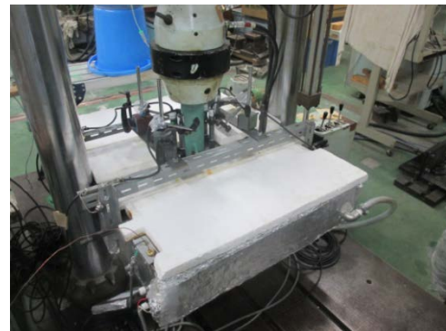
Fig.4 Fatigue test setup
