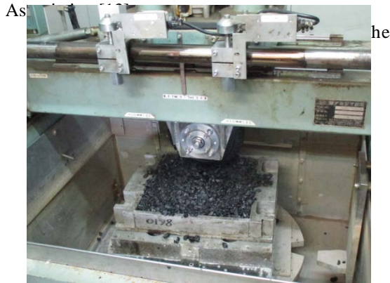
Fig.8 Aggregate fretting test
