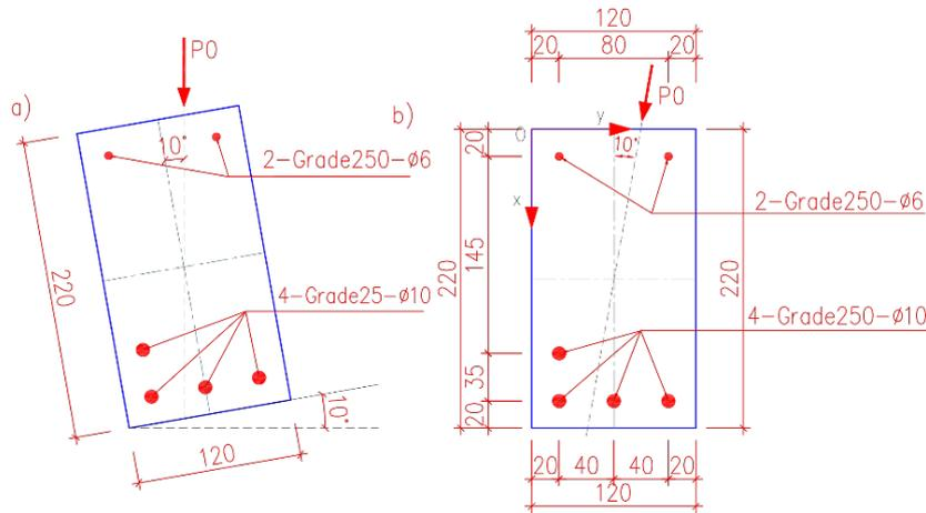
Fig. 2. Cross-section of the reinforced concrete beam, a) rebar layout, b) dimensions in detail
