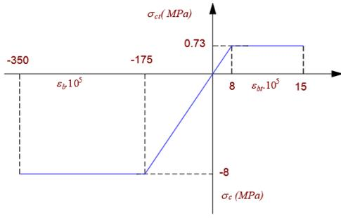
Fig. 3. Bilinear stress-strain relationship of concrete
