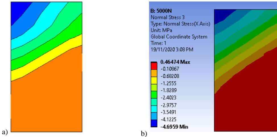
Fig. 15. Stress spectrum on the cross-section for case 2
