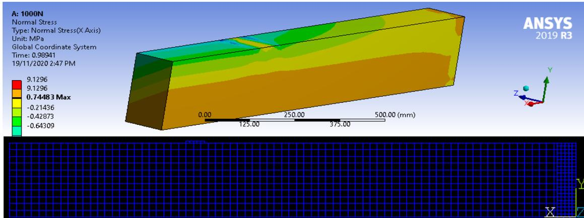
Fig. 10 Stress spectrum of case 1 ( $M=106$  N) and cracks along beam length
