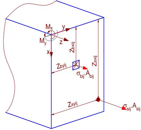
Fig. 5. The cross-section shows the parameters of concrete and reinforcement elements.
