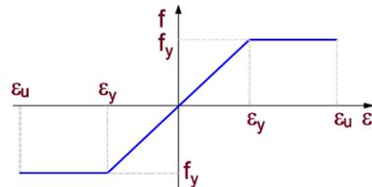
Fig. 9. The stress-strain relationship of reinforcement
