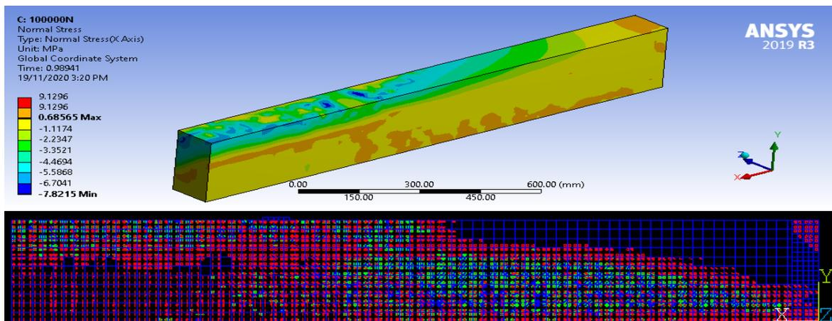
Fig. 12 Stress spectrum of case 3 ( $M = 5.106$  N) and cracks along beam length
