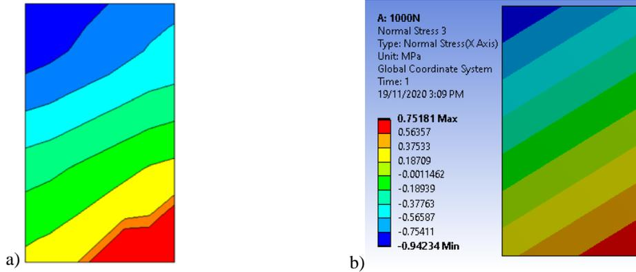
Fig. 14. Stress spectrum on the cross-section for case 1
