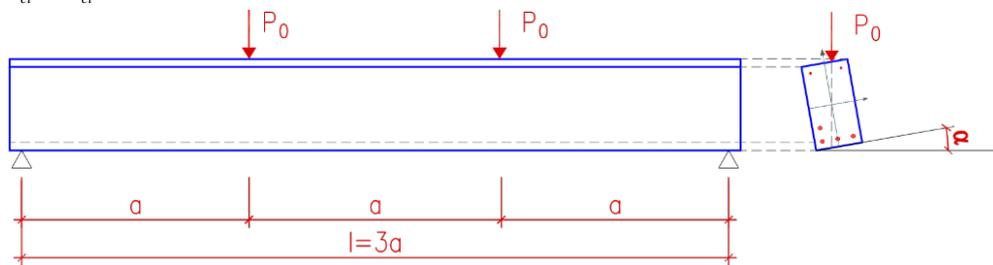
Fig. 1. Model of the reinforced concrete beam for biaxial bending
