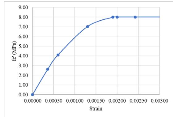
Fig. 8. The relationship of stress - deformation state of concrete
