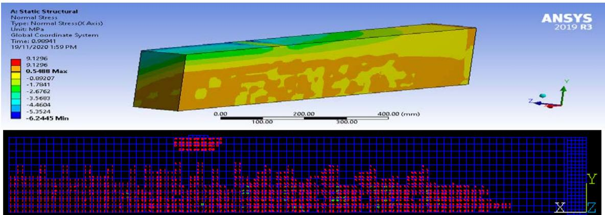
Fig. 11 Stress spectrum of case 2 ( $M=5.106$  N) and cracks along beam length
