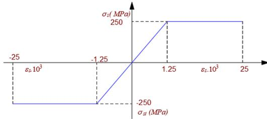
Fig. 4. The bilinear stress-strain relationship of the reinforcement
