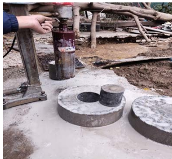
Fig. 4 Drill sample to test concrete abrasion
