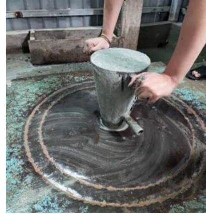
Fig. 2 Slump flow test (Inverted Mold)
