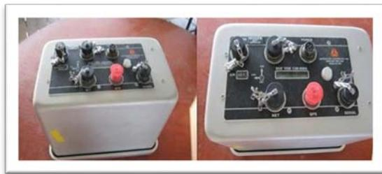
Fig.2 Accelerometer equipment Model version 130-SMA
