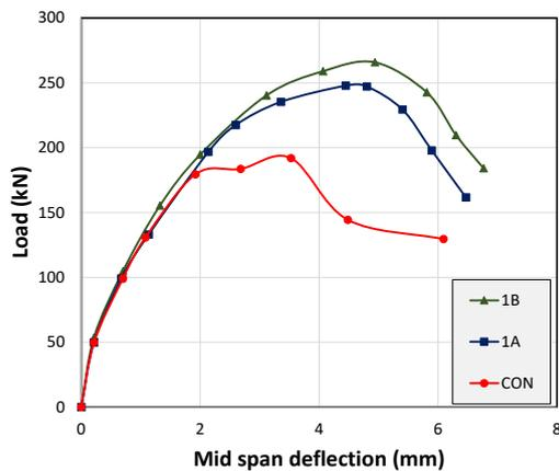
Fig.6 The load-deflection response of beams in group 1 and 2
