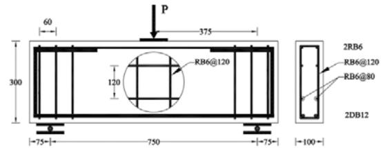
Fig.1 Typical detail of test specimen (unit in mm)
