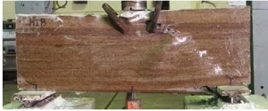
Fig.10 Failure mode of beam 1-B
