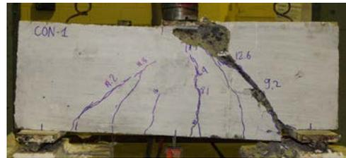
Fig.8 Failure mode of control beam
