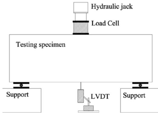
Fig.5 Loading setup
