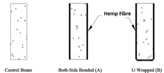
Fig.2 Details of strengthening configuration
