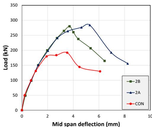
Fig.7 The load-deflection response of beams in group 1 and 2
