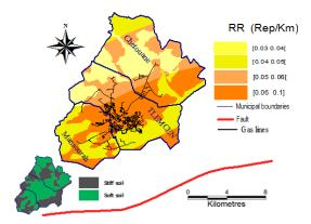
Fig. 8 Map of the mean predicted RR (using the models 4) for the city of TLEMCEN for a scenario earthquake of M =6.5 occurring on the southern fault (red line).
