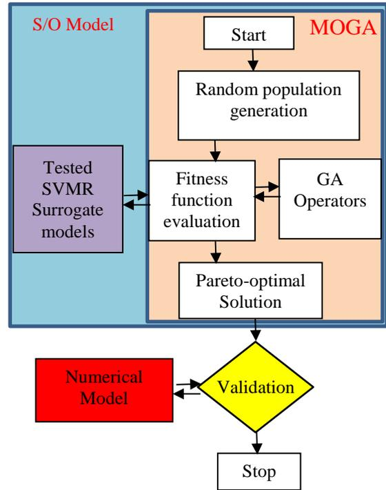
Fig. 2 Flowchart for the linked S/O model with optimal solution validation stage
