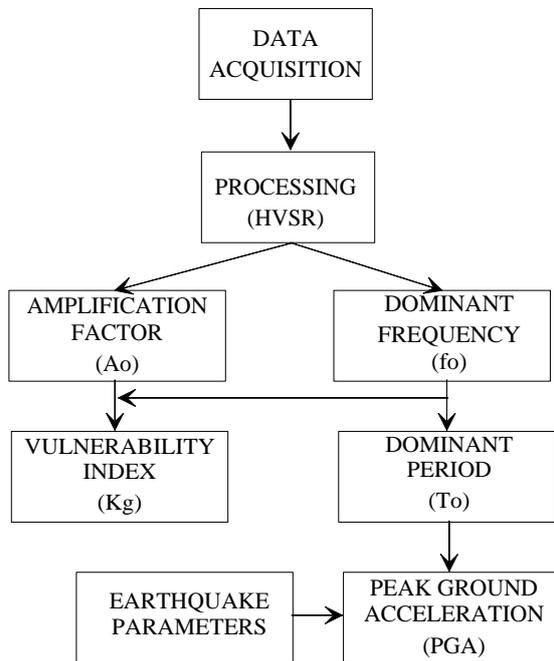
Fig. 2. Flowchart of data processing
