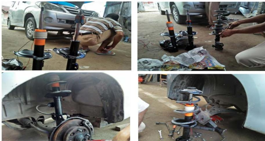
Fig.15 Installing the regenerative shock absorber in the car
