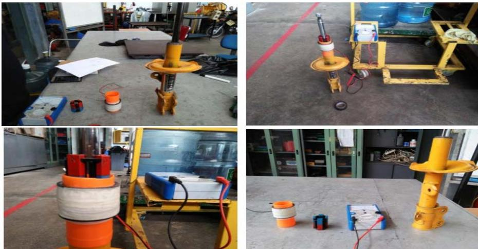
Fig.14 Shock absorber with harvesting energy mechanism
