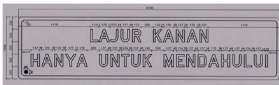
Fig. 7 Dimension of two line Road Sign due to FHWA 1977 Resource: TRBM Management
