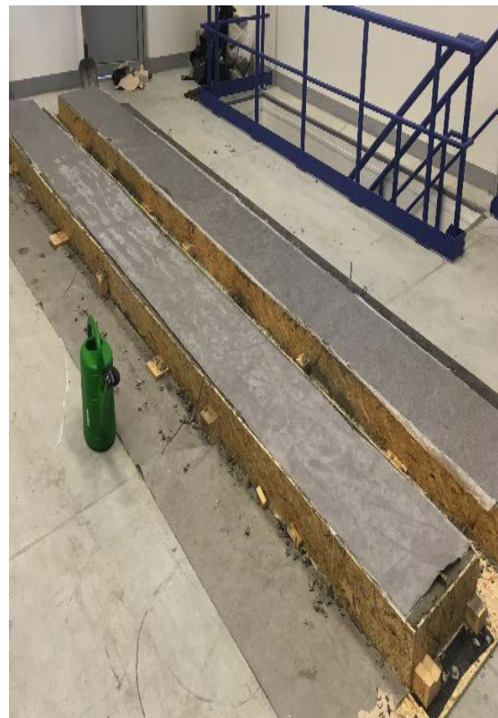
Fig. 3 Large-dimensional specimens in laboratory during concrete curing
