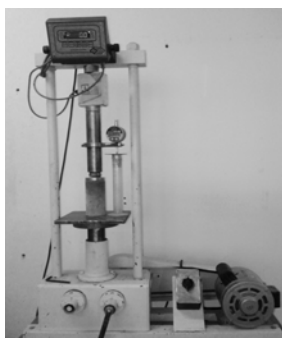
Fig.2 Marshall press machine for unconfined compression tests
